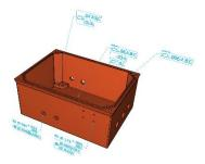
3D geometric data, tolerances, PMI dimensions, assembly, attributes and UUIDs (Universally Unique Identifiers) are available with QIF to PDF, QIF to JT and QIF to STEP convertors.
